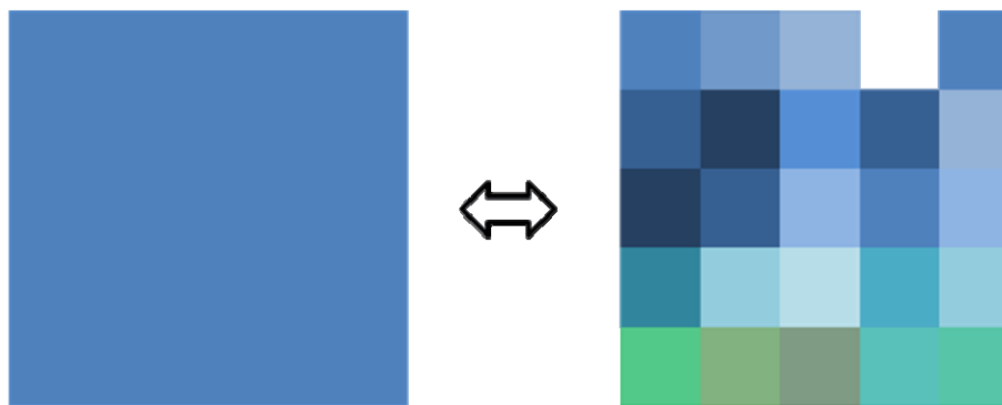
Fig. 1. (left) A pixel observed by a low-resolution sensor; (right) Pixels observed by a high-resolution sensor, corresponding to the low-resolution pixel.
