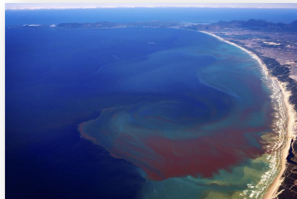
Fig. 4. A part ( 37.6 \times 57.2 km) of a true color image advanced Land Imager (ALI) acquired on 14 July 2002 in the western part of the Gulf of Finland. Areas in which pres surface scums was estimated using band 4 (775–805 nm) refl values are shown in red. The Hyperion footprint seen in F indicated with the frame.
