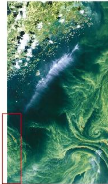
Fig. 4. A part ( 37.6 \times 57.2 km) of a true color image advanced Land Imager (ALI) acquired on 14 July 2002 in the western part of the Gulf of Finland. Areas in which pres surface scums was estimated using band 4 (775–805 nm) refl values are shown in red. The Hyperion footprint seen in F indicated with the frame.
