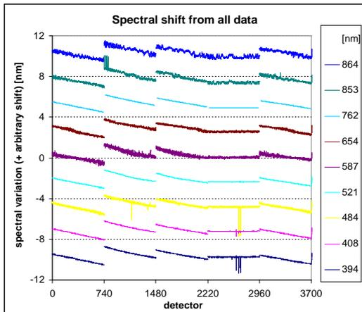
On- Orbit Spectral characterisation measurements (Erbium Doped diffuser, Fraunhofer lines, O2-A)
