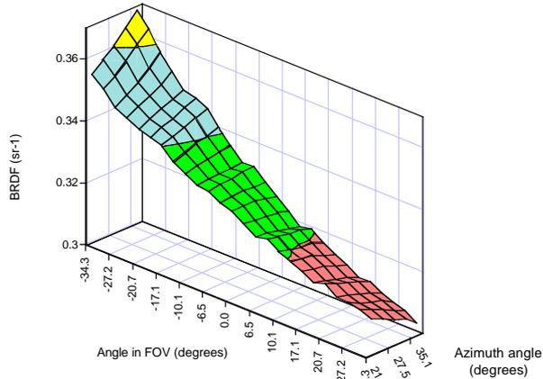
On-ground characterisation of diffuser-1 @ 410nm
