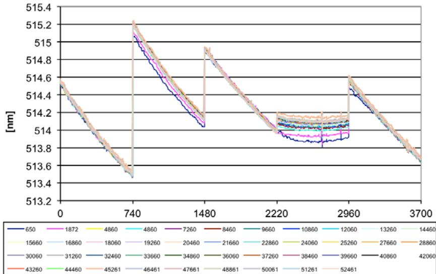
Spectral calibration using Erbium doped diffuser, row #9 ca. 400 nm, all orbits
