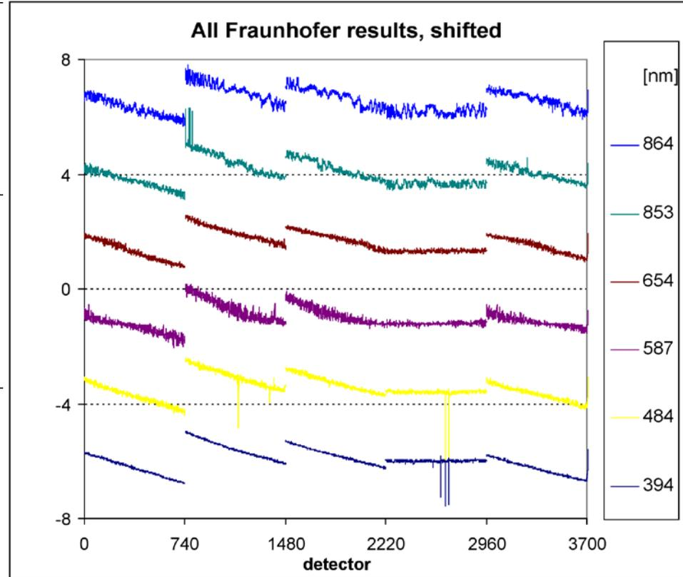
Method: Spectrum-matching, with correction for Air-Vacuum (Edlen)
