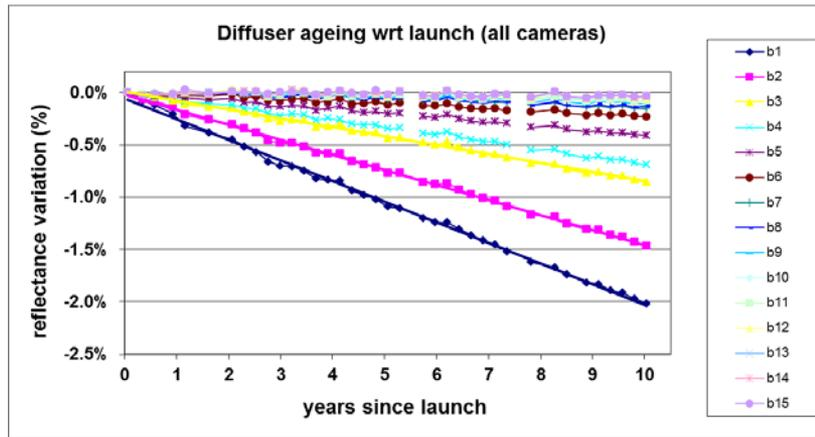
Diffuser Degradation process is linear
