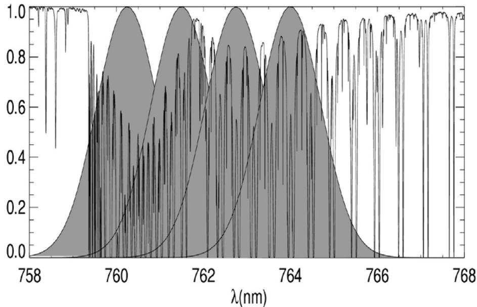
Oxygen O2A absorption spectrum
