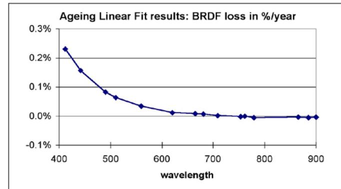
Diffuser Degradation rate per year
