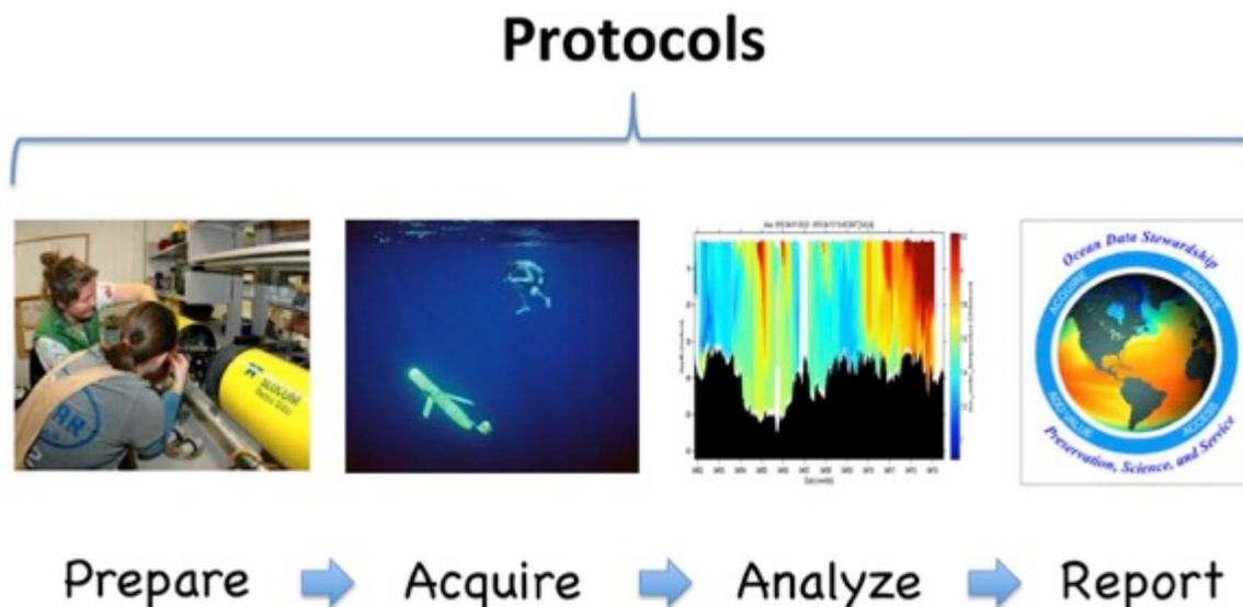
*Figure 2. Expanded concept of ocean optics protocols encompassing instrument preparation, deployment and data acquisition, quality assurance based on post deployment sensor calibration and the assignment of quality flags, and reporting with metadata that provides accurate descriptions of the data and insures ease of discovery.*
