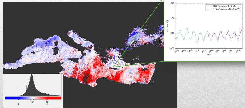
Impact of vicarious calibration on chlorophyll-a concentration, as measured by MERIS over the Med Sea in April 2008. The relative change (in %) is due to disabling vicarious calibration.
