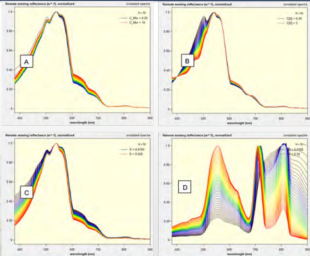
Figure 1: Normalized remote sensing reflectance for (A) TSM range 0.2 - 10 mg/l, (B) CHL range 0.2 - 5  $\mu\text{g/l}$ , (C)  $S_{CDOM}$  range 0.010 - 0.020  $\text{nm}^{-1}$ , (D) depth range 0.01 - 0.5 m.
