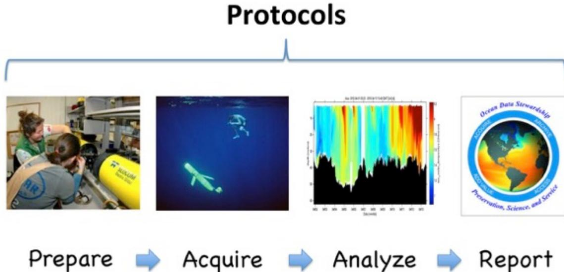
*Figure 2. Expanded concept of ocean optics protocols encompassing instrument preparation, deployment and data acquisition, quality assurance based on post deployment sensor calibration and the assignment of quality flags, and reporting with metadata that provides accurate descriptions of the data and insures ease of discovery.*
