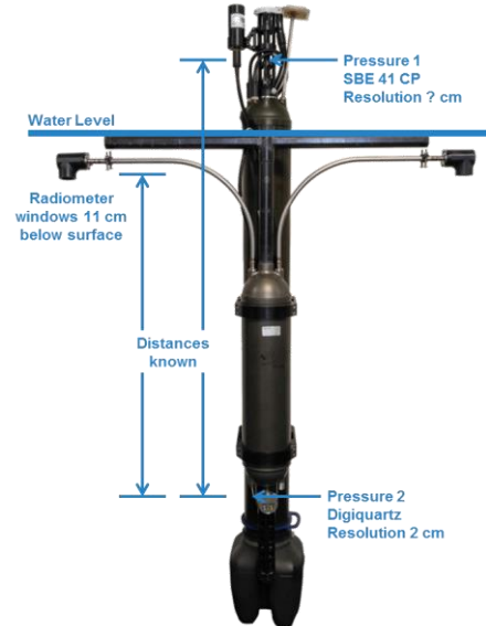
HyperNav system - Navis float, Hyperspectral L_u \times 2
