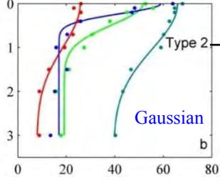
$$f_2(z) = C_0 + \frac{h}{\sigma\sqrt{2\pi}} \exp\left[-\frac{1}{2}\left(\frac{z-z_0}{\sigma}\right)^2\right]$$
