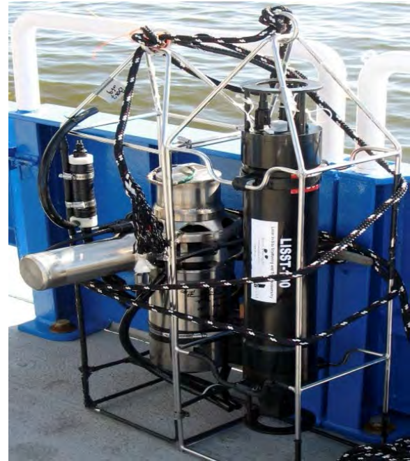
Multi-Spectral Volume Scattering Meter (MVSM), NRL. Measurements of the hydrosol volume scattering function in the range of 0.5-179 deg.
