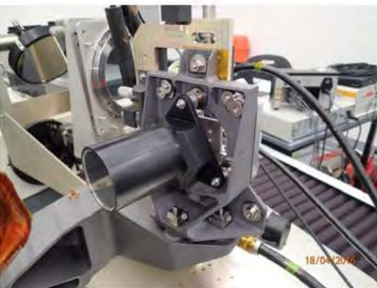
Focal grid and tool with DCW FLW alignment
