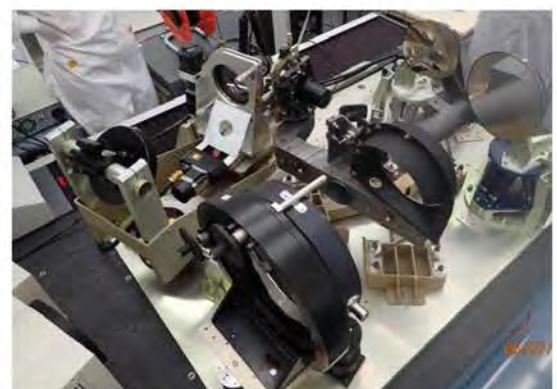
Interferometer setup and ACFlat alignment
