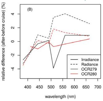
Relative difference of calibration coefficients determined at the LOV calibration laboratory before and after deployment
