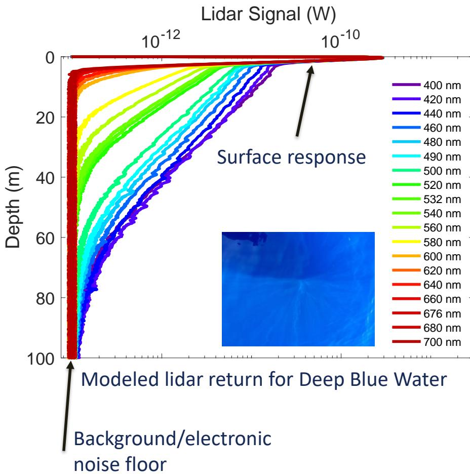
Modeled airborne lidar signals showing spectral returns as a function of depth
