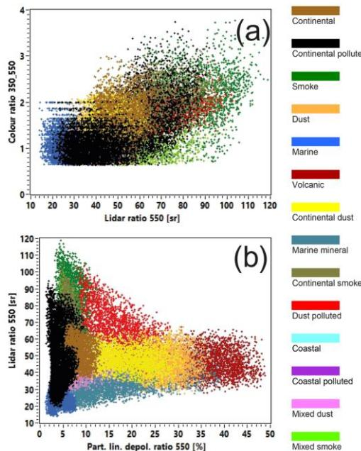
Work with European Aerosol Research Lidar Net- work (EARLINET) data show aerosol discrimination using a three wavelength approach
