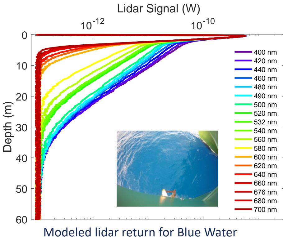
Modeled airborne lidar signals showing spectral returns as a function of depth
