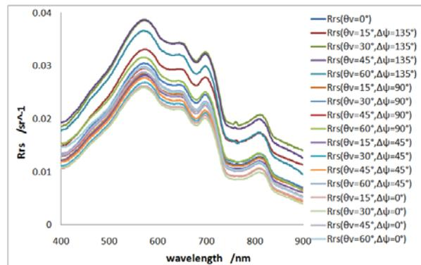
Fig. 1 Multi-angle remote sensing reflectance spectra on a typical sampling site. (Where  $\theta_v$  is viewing zenith angle;  $\Delta\psi$  is relative azimuth angle, which is the difference between viewing azimuth angle and solar azimuth angle, and  $\Delta\psi$  is  $0^\circ$  if the sensor and the sun are in the same direction from the target.)
