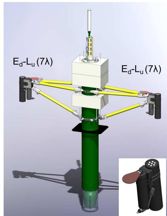
*The ProVal float with 2  $E_d-L_u(7\lambda)$  combo*
