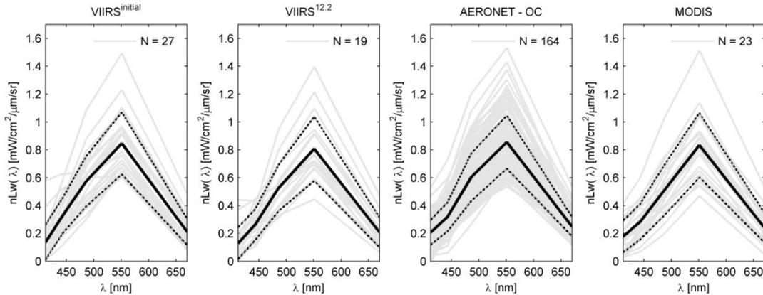
Figure 1.  $nLw(\lambda)$  match-up spectra of VIIRS<sup>initial</sup> (1<sup>st</sup> column), VIIRS<sup>12.2</sup> (2<sup>nd</sup> column), SeaPRISM (3<sup>rd</sup> column) and MODIS (4<sup>th</sup> column) for the LISCO site.  $N$  is the total number of spectra for each sensor. Grey lines represent the individual spectra. Thick black solid lines indicate average and thick dashed lines indicate  $\pm$  one standard deviation).
