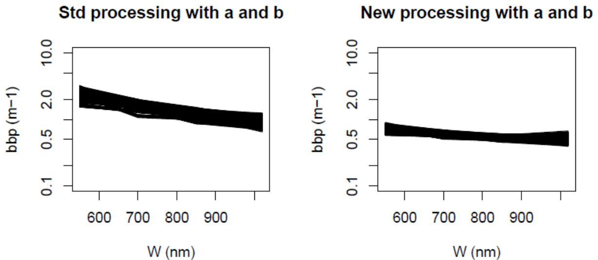
*Fig. 1: Particulate backscattering coefficient spectra ( $b_{bp}$  in  $m^{-1}$ , 550 – 1020 nm) measured in the Río de la Plata estuary using a HydrosCat-4 sensor (HOBI Labs). Comparisons between results (spectral  $b_{bp}$  values) obtained using the standard (left) and new processing (right).*
