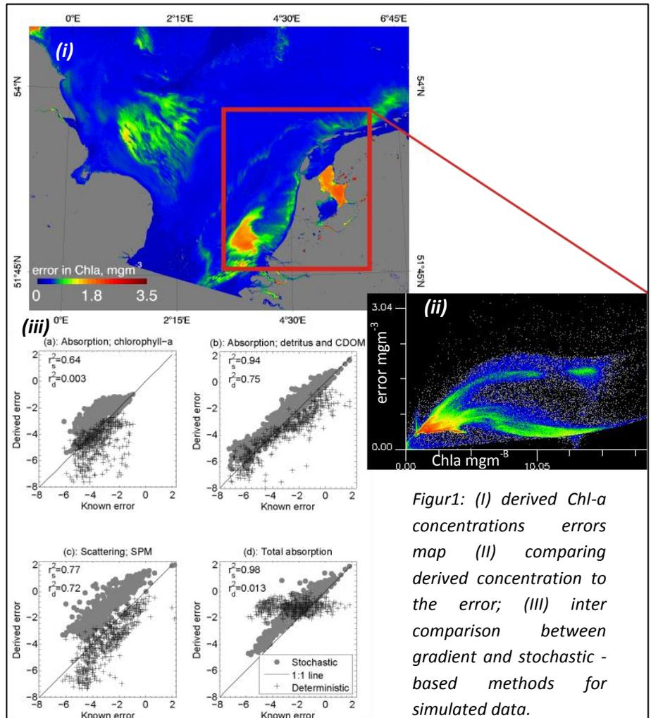
Figur1: (I) derived Chl-a concentrations errors map (II) comparing derived concentration to the error; (III) inter comparison between gradient and stochastic-based methods for simulated data.
