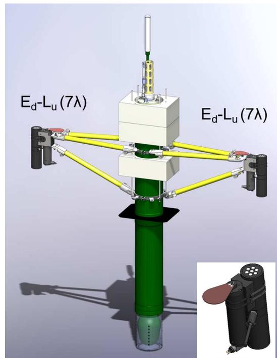
*The ProVal float with 2  $E_d-L_u(7\lambda)$  combo*
