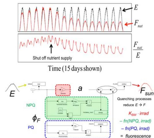
Fig. 1. Top: Laboratory data showing the degree of dynamical complexity in daily  $F_{nat}$  for 15 days before & during nutrient starvation. Daily trends in  $F_{nat}/E$  can be explained by a dynamical model (bottom) of daily irradiance  $E$  which predicts daily  $F_{sun}$  trajectories with only a few parameters.
